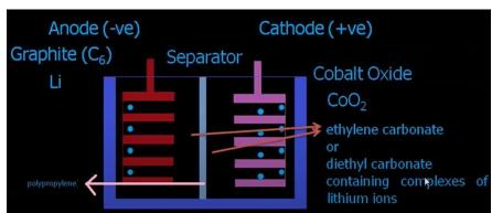
In lithium-ion battery, the anode is made up of layered of graphite which is intercalated (inserted) with lithium, the cathode is made up of cobalt dioxide ( $CoO_2$ ), these two electrodes are dipped in an electrolyte containing LiPF<sub>6</sub> (Lithium hexafluorophosphate) dissolved in ethylene carbonate or diethyl carbonate, these two electrodes are separated microporous poly propylene separator.
