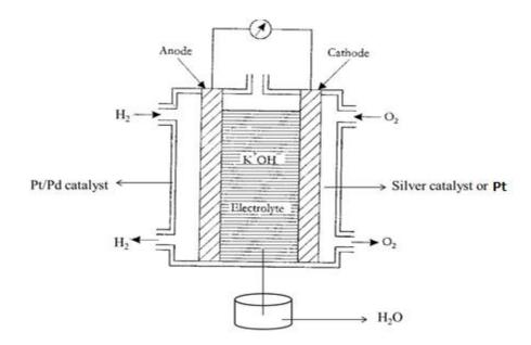
In this H<sub>2</sub> - O<sub>2</sub> fuel cell, hydrogen gas is used as a fuel and oxygen gas is used as oxidant. The
