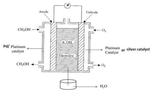
In this Methanol-  $O_2$  fuel cell, Methanol is used as a fuel and oxygen gas is used as oxidant. The Methanol-  $O_2$  fuel cell consists of two electrodes made of porous Ni. The anode is coated with finely divided platinum or palladium catalyst. The cathode is coated with platinum or silver catalyst. These two electrodes are placed in aqueous solution of KOH (30 %), which acts as electrolyte.
