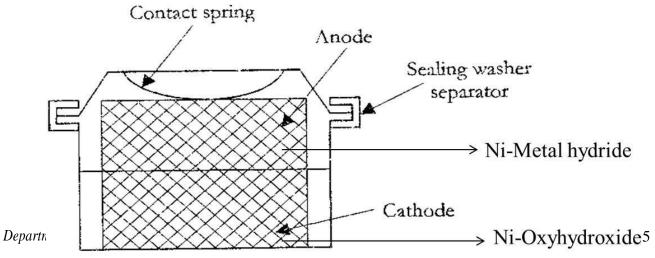
It consists of rectangular nickel wire gauze grids. The anode grid is coated with a metal-hydride as the active material, while the cathode grid is coated with nickel oxyhydroxide. The anode and cathode grids are separated by a microporous polypropylene separator. Both electrodes are immersed in a 21% KOH solution, which acts as the electrolyte.
