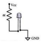
The LED is a p-n junction diode, made up of semiconductors. LED is an output device for visual indication in any electronic device. LED can be interfaced to the port pins of a microcontroller in the following way:
