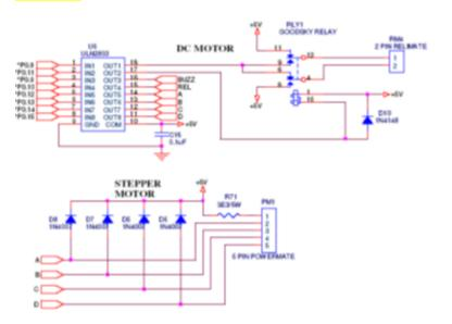
/\* A stepper motor direction is controlled by shifting the voltage across the coils. Port lines: P0.12 to P0.15\*/
