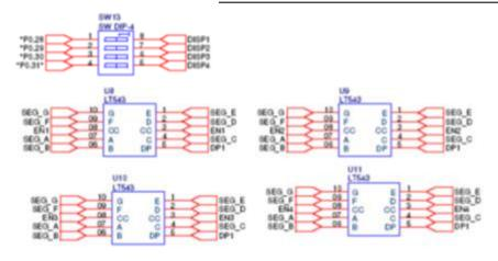
Keep all pins of SW13 in ON position and un short the jumper JP21. Short jumper JP2/1-2
