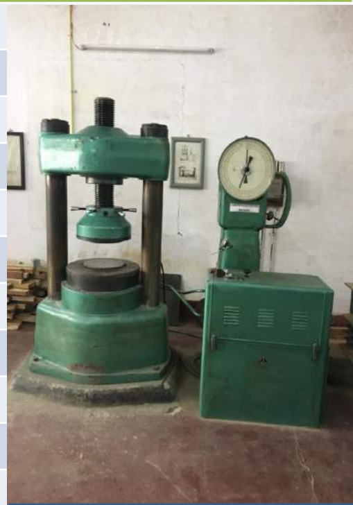
200 ton compression Testing Machine in BMT Lab
