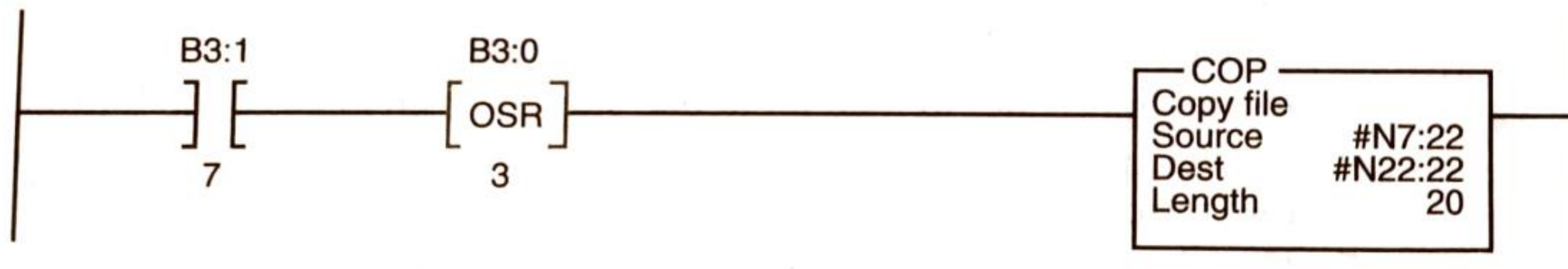
Figure 13-13 Internal bit B3:0/3 controlling a one-shot instruction to enable data to be copied only once per trigger of bit B3:0/3.
