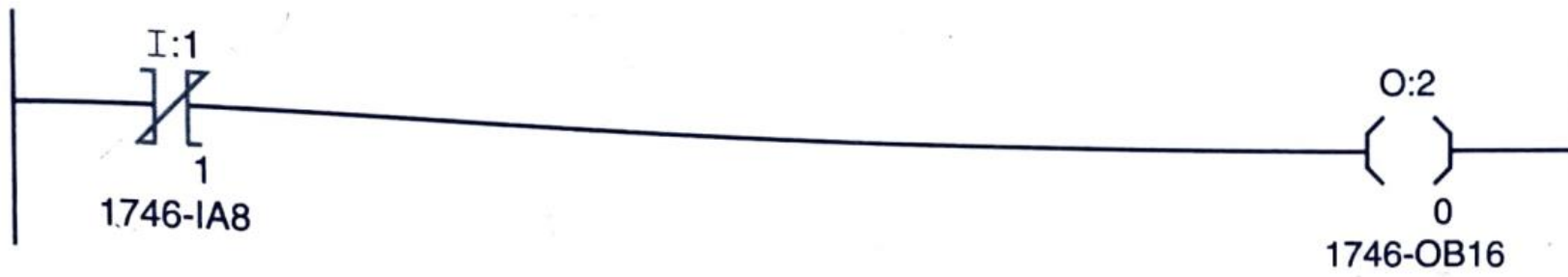
Figure 13-8 Normally closed, or examine if open, instruction controlling an OTE instruction.
