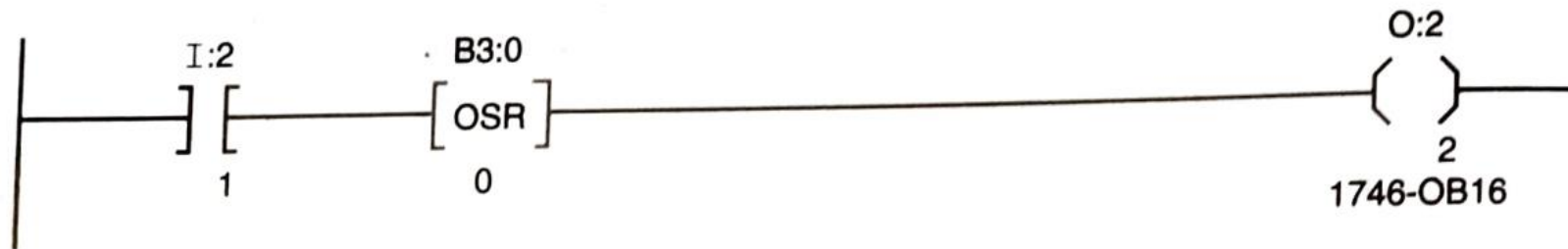
Figure 13-10 SLC 500 family one-shot ladder rung.
