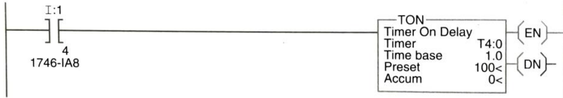
Figure 16-1 SLC 500 on-delay timer.
