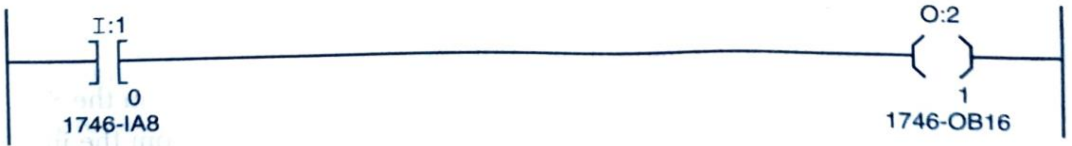
Figure 13-3 Ladder rung containing an examine if closed input instruction and an output enable instruction.
