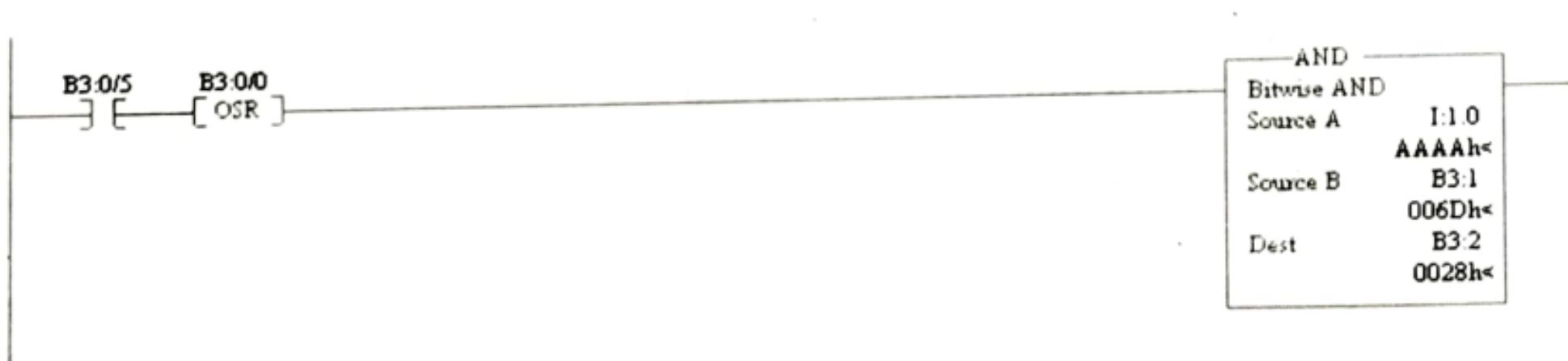
Figure 17-26 RSLogix 500 software AND instruction.
