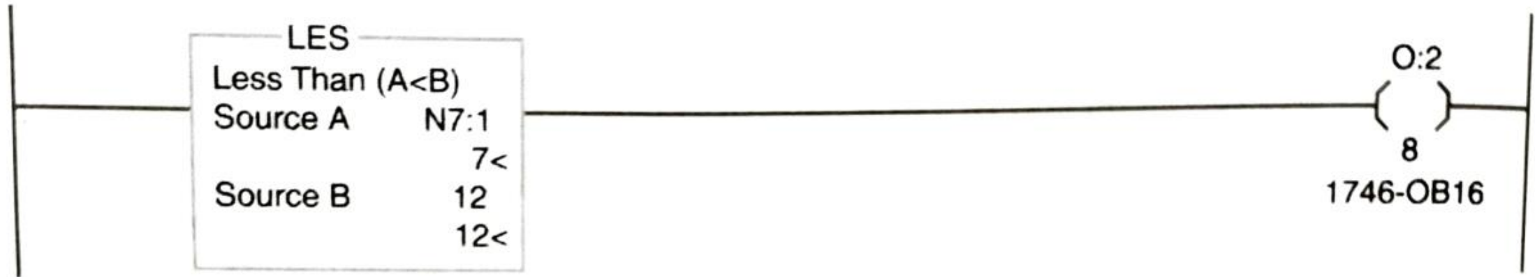
Figure 17-3 The less than instruction tests to see if the value in source A is less than the value stored in or addressed as source B.
