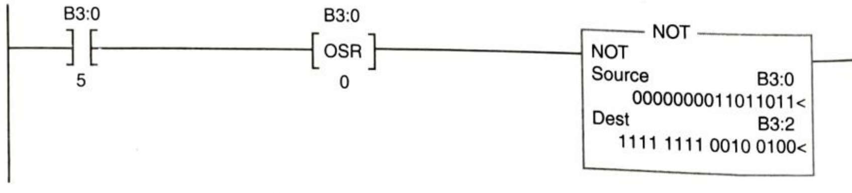
Figure 17-37 NOT logic as an output instruction on a PLC ladder rung. After execution, destination will contain 1111 1111 0010 0100.
