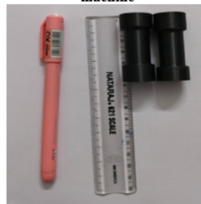
Tensile test samples coated by 3D printed samples
