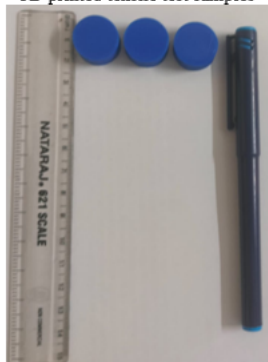
3D printed compression & hardness test samples
