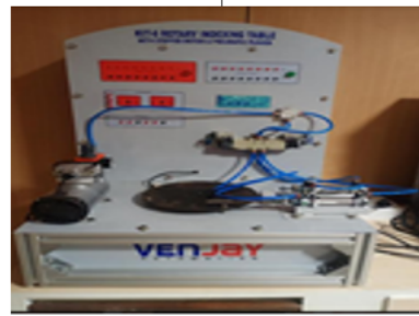
Rotary indexing table with stepper motor and pneumatic pusher Training Setup
