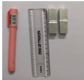
Impact test samples prepared by CNC machine
