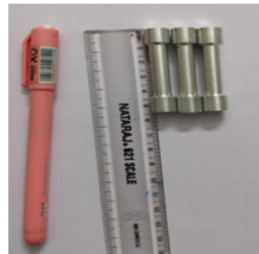
Tensile test samples prepared by CNC machine
